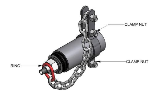
WHEN PROPERLY INSTALLED, ACCORDING TO OUR INSTRUCTIONS, THE **THAXTON PIPE STOPPER** IS A SAFE TOOL THAT WILL GIVE MANY YEARS OF SATISFACTORY SERVICE. HOWEVER, AS AN EXTRA SAFETY FACTOR, WE RECOMMEND USE OF A SAFTEY GAG. IT SHOULD BE INSTALLED AFTER THE PLUG IS IN PLACE AND BEFORE PRESSURE IS ADDED.
